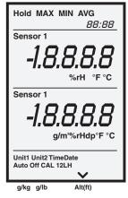
arrow on the screen above the Alt. (ft) label on the case. Move the wheel up and down to adjust the altitude. You can adjust the altitude with  $\triangle$  and  $\nabla$  and confirm by  $\triangleright$ .
